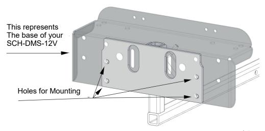
The only assembly required will be to insert the long tube into your hitch receiver on your vehicle. Secure in place with a 5/8" diameter pin (Not Included).
